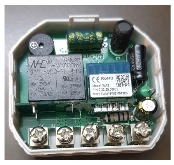
As mentioned above, to make it work with tasmota the Beken chip module has to be replaced with an ESP module (ESP12E used here, but probably any of the ESP modules would do.) You will need a steady hand, tools for soldering, some additional cutting tool (like dremel), some wires, 10K resistance, knife and maybe some tool to tear off isolation from the wires. After the procedure described below, the module will look
